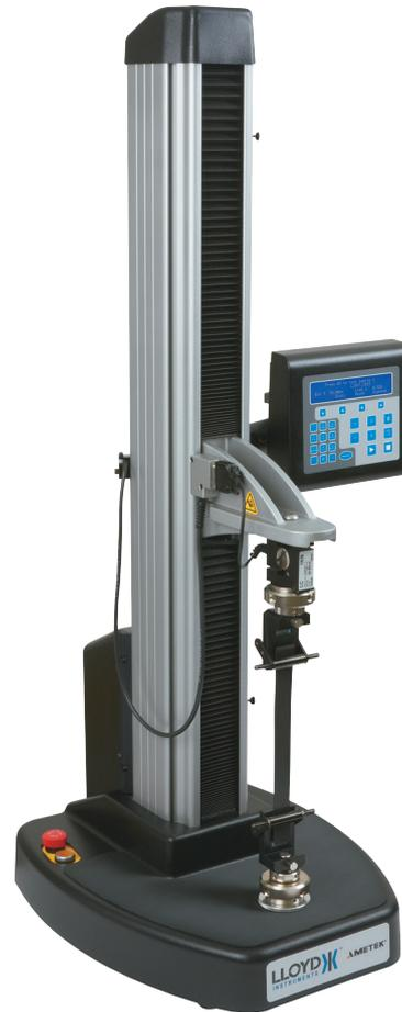
The LS5 is a 5 kN / 1124 lbf high precision material testing machine that combined with our extensive range of grips, fixtures, extensometers and software creates a powerful material testing system. The system is equally suited to quality control, educational and R&D environments within a wide range of applications and test types, including medical devices, plastics, packaging, textiles, rubber and electronics to name a few.
